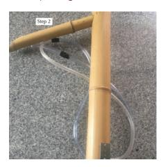
2. Loosen the two screws using a screwdriver, twist the metal spike so that it is facing downwards and place the screws back in the top and bottom holes.
